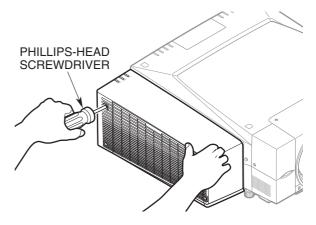
**6** Check that the Smoke Resistant Box is fixed in place with the four screws and no wide gap exists between the projector body and the box.
